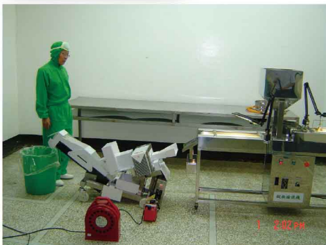
MD0903A Slide-down Channel w/ Electric Reject Device + Adjustable Height & Angle Tilt
