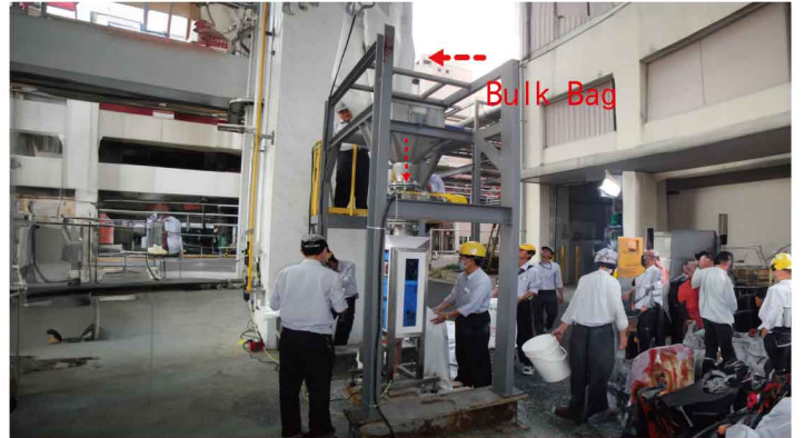
氣密直落式金檢機檢測寶特瓶塑料內金屬異物 MD1212 Gravity Sealed Detection Channel for testing plastic bottles
