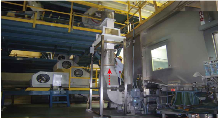
管通式金檢機檢測化纖棉內金屬異物 MD4520 w/ rising up tube for testing cotton
